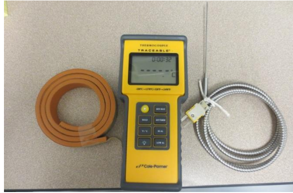
from left: cell foam tape, thermometer and needle tip probe
