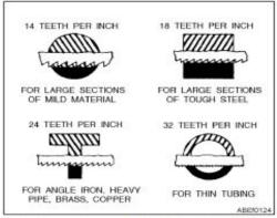
Figure 1-14.—Selecting the proper hacksaw blade.
