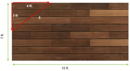
If the third measurement is 5, you know the corner is square. If it is not 5, ensure the measurements of the two sides are 3 and 4.
