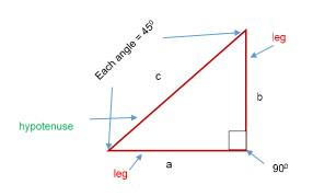
In a right-angle triangle, the length of the  $(hypotenuse)^2$ is equal to the sum of (side a)<sup>2</sup> and (side b)<sup>2</sup>.
